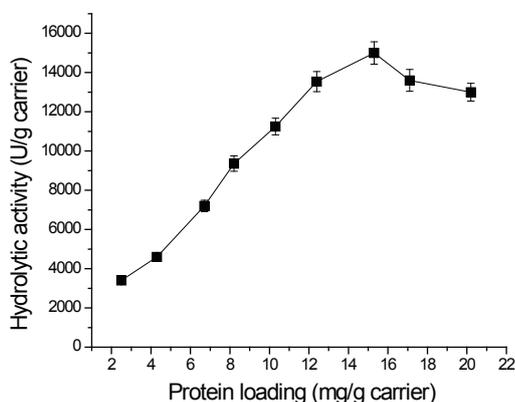
Fig. 1. Effect of the amount of loaded protein on the activity of nanoSnO<sub>2</sub>-MC7.
