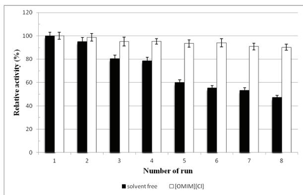
Fig. 5. Multiple use of nanoSnO<sub>2</sub>-MC7 in stearyl stearate synthesis.
