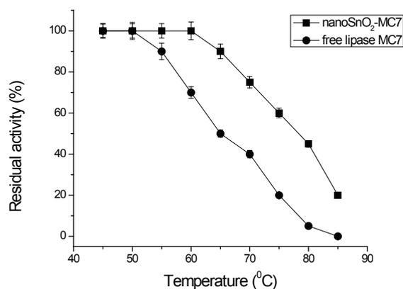
Fig. 2. Effect of immobilization on thermal stability of lipase MC7.
