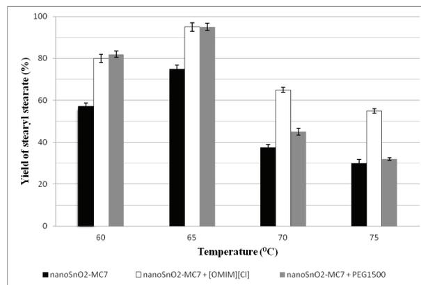
**Fig. 4.** Effect of the reaction temperature and additives on stearyl stearate synthesis catalyzed by nanoSnO<sub>2</sub>-MC7.
