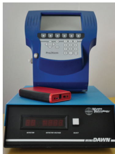
Fig. 1. Light-scattering evolution showing the traditional market leader (bottom), original AggreKem with built in PC (top), and PAM Zero (front). Reprinted with permission from White et al. (6), Mechatronics and Manufacturing Engineering: Research and Development , Woodhead Publishing Ltd., ISBN 0 85709 150 6.
